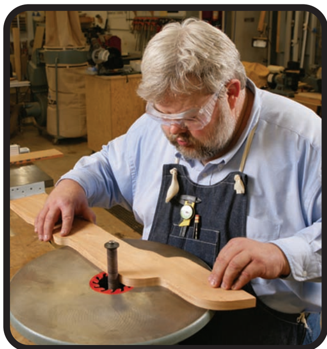
To remove the saw marks, and even to help shape some of the curves, a spindle sander is a very handy tool on this job.
