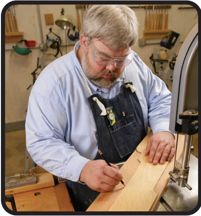
Create templates of the shaped parts from the gridded drawings on pages 46 to 49. Use the templates to transfer the shapes to each piece as needed.
