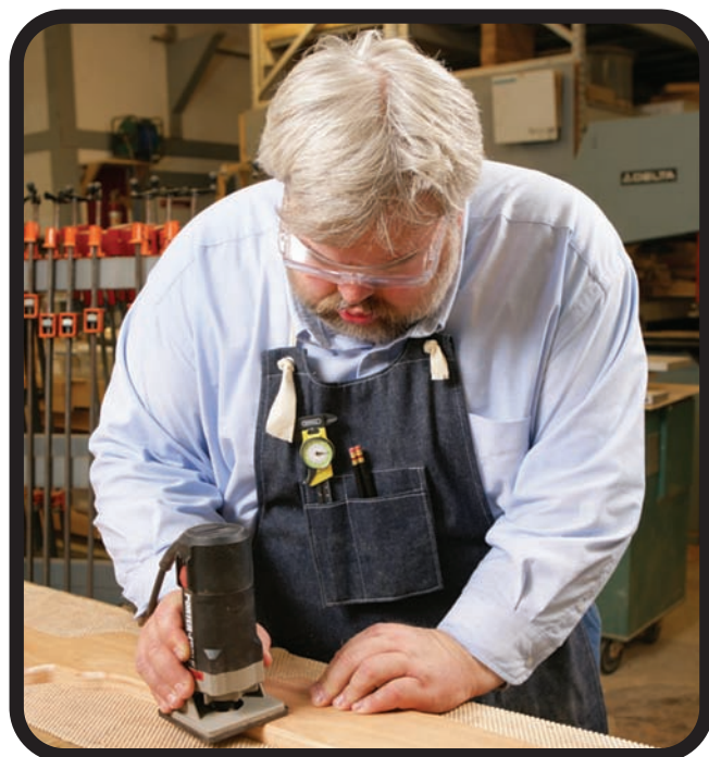
Use a trim router equipped with a 1/4" roundover bearing-guided bit to soften the chair's organic shapes.
