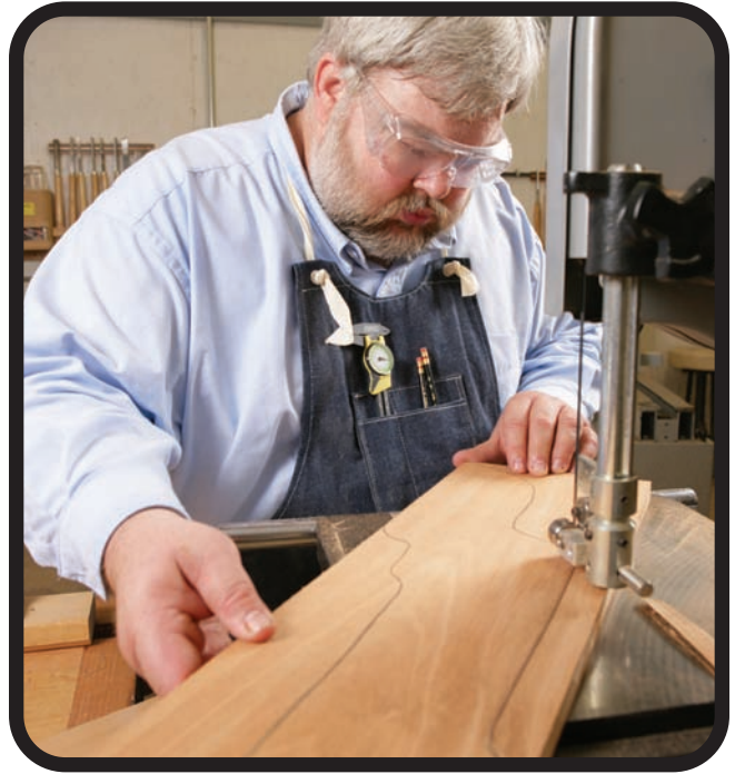
Shape the parts using a band saw with a 1/4" blade. Some of the cloud lifts and curves require tight corners to be cut.
