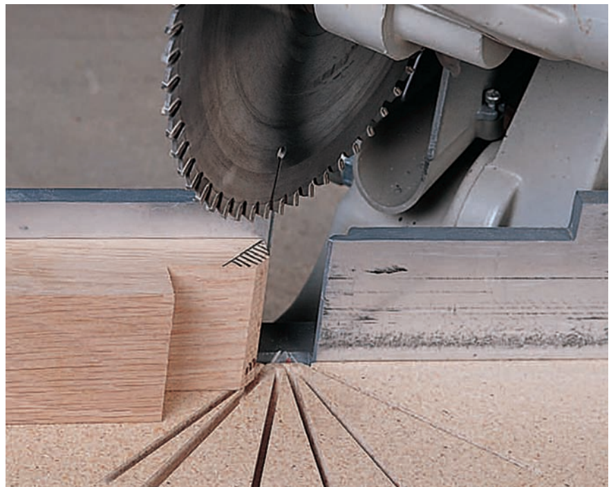
Figure 2: Cut the 45° miters on the bottom aprons using a miter saw. Nibble at the cut to prevent your saw from flinging small pieces of oak across the room.
