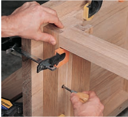
Figure 5: With the top firmly clamped to the aprons, tip the bench on its back and mark the locations of the pilot holes with an awl.
