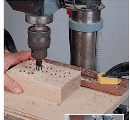
Figure 6: You can cut your own screw hole plugs with a 3/8" plug cutter in your drill press. Cut the plugs loose by resawing to 3/8" on your band saw.
