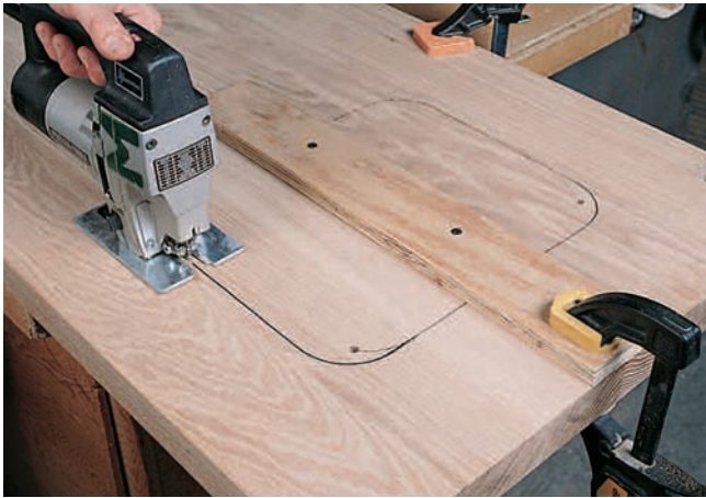
Figure 3: Cut the mixing tub hole to shape with a jigsaw. Cut three sides of the hole, then screw a holding bracket to the waste so it doesn't pinch your blade or fall out while you cut the fourth side.
